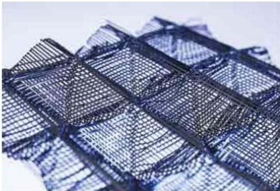
AMOL 55-Advanced technical textile web tested on the Monforts TT-Range
