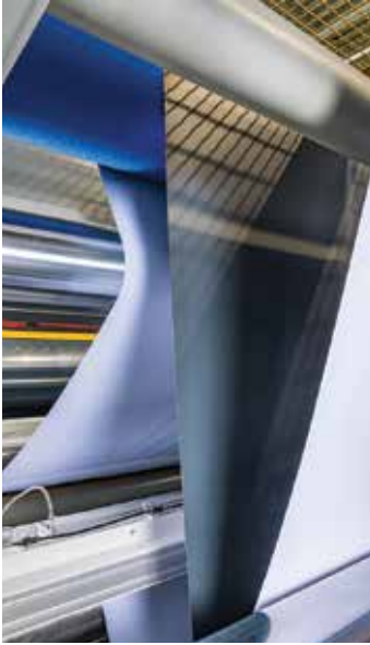
▼ The substrates of choice for digital printing are 100% polyester warp knits which have extremely smooth surfaces.
