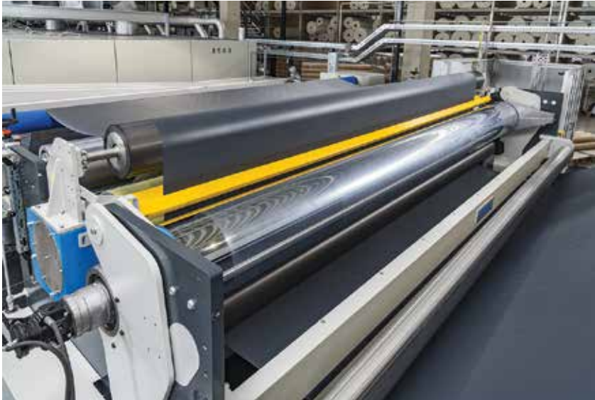
▼ GtA now finishes rolls in sizes of between 1,500 and 2,000 metres directly on the Monforts stenters.
